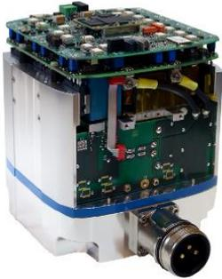
Electrolytic capacitor-less single-phase to three-phase SiC AC/ AC Integrated Motor Drive System (IMDS).
