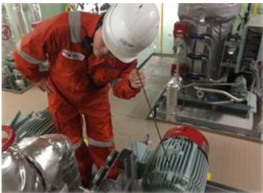
Checking sound using a typical listening rod
