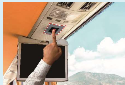
Emergency Driving Stop System (EDSS) that can be attached as an additional component
