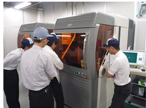
Research on quality improvement conducted at CMET Inc. Optimization of the stereo lithography conditions by quality engineering
