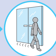
Doors equipped with the Intelligent eco Door System will not open when a person passes by.
